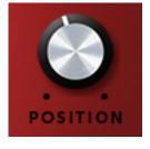
When you turn of insert mode, Mikron Reverb will be treated as a send effect. In this case the dry/wet mix will be always 100%. The position knob will still determine the early/late mix, but if you want the dry/wet mix to reflect the position of the listener in the room as well, you will have to tune it that way yourself through the send.
