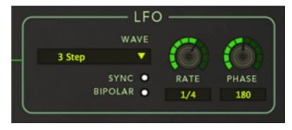
Hold. You can set the amount with which the LFO affects its destination with the mod knobs in the sections above. All knobs on zero means the LFO will do nothing.
